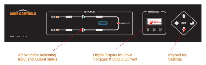
**Digital Display**: Three-digit seven-segment digital display indicates the AC Voltage of INPUT-A, AC Voltage of INPUT-B and the Output load Current.
