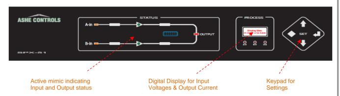
**Digital Display**: Three-digit seven-segment digital display indicates the AC Voltage of INPUT-A, AC Voltage of INPUT-B and the Output load Current.
