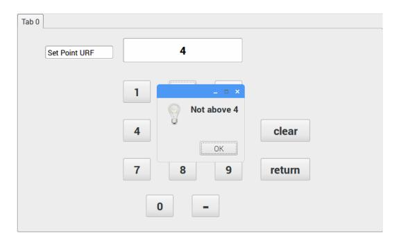
In this window we can set the set point of Under Range Fault.
