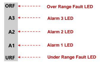
The three Red LEDs A1, A2 and A3 indicate the three Gas alarm level for individual channels.
