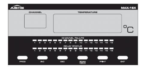
The Temperature Scanner has two display windows on the front panel - a four-digit display indicating the temperature value and another two-digit display for indicating the channel number.
